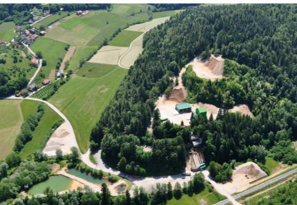
With an annual extraction of 35,000 t of quartzite, the site Mirna supplies our factories in Svitavy and Dr. C. Otto in Bochum with the best premium refractory quartzite for the production of our refractory products.
